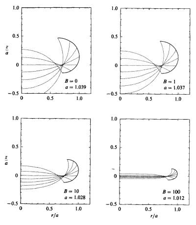
FIGURE 4. Meridian of container (solid curve) for contact angle 60° and several Bond numbers showing meridians of some symmetric equilibrium solution surfaces (dashed curves), all having the same contact angle and energy, and enclosing the same volume of liquid.
