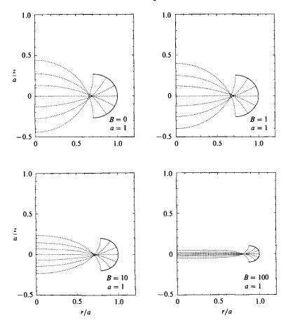
FIGURE 5. Meridian of container (solid curve) for contact angle 90° and several Bond numbers showing meridians of some symmetric equilibrium solution surfaces (dashed curves), all having the same contact angle and energy, and enclosing the same volume of liquid.
